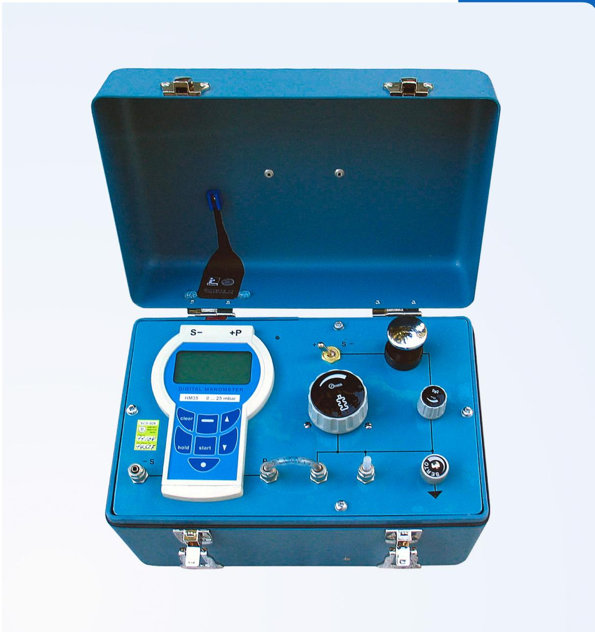
In this handy calibrator a digital manometer of the Swiss producer HUBER AG with the distinction of high precision, temperature compensation and long-term stability is built in. Pressure is generated by the integrated hand pump, the variable bellows serves fine pressure tuning and precise generation
